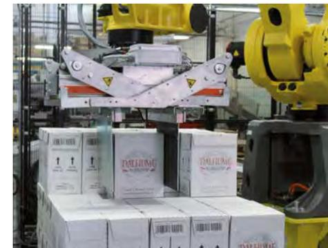
If used as a cartoning/boxing machine, on the other hand it will be equipped with bottle pick-up heads, fixed or adjustable, depending on customer requirements. An important and recent innovation is the **automatically adjustable head**, that can be used to process many types of bottles with different
